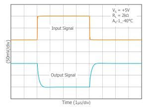
$T_A = 25^{\circ}C$ ,  $V_S = +5V$ ,  $R_f = R_g = 10k\Omega$ ,  $R_L = 10k\Omega$  to  $V_S/2$ , G = 2; unless otherwise noted.
