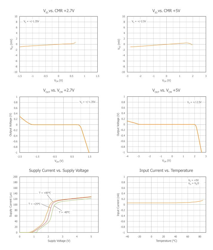
$T_A = 25^{\circ}C$ ,  $V_S = +5V$ ,  $R_f = R_g = 10k\Omega$ ,  $R_L = 10k\Omega$  to  $V_S/2$ , G = 2; unless otherwise noted.
