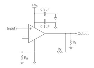
Figure 4. Single Supply Non-Inverting Gain Circuit
