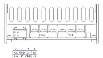
Vout terminals are rated for 25 A max. At higher current connection has to be splitted.
