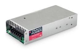
The TXH 600 series models are very compact 600 Watt universal power supplies. Rear side IEC-C13 line socket including mains switch and fuse and the output screw terminal make the connection of these power supplies very easy. Sense line, auxiliary output, remote control, adjustable output voltage, and load share line for up to 3 units in parallel make the units all-purpose applicable.
