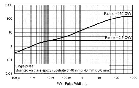
TRANSIENT THERMAL RESISTANCE vs. PULSE WIDTH
