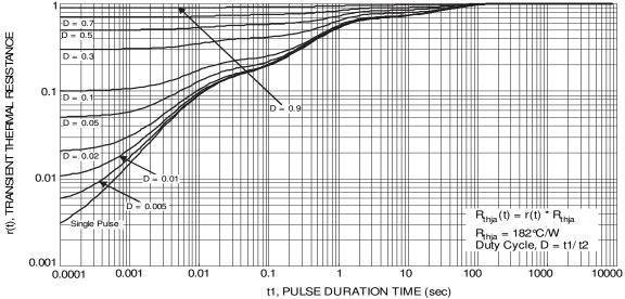
Figure 13 Transient Thermal Resistance
